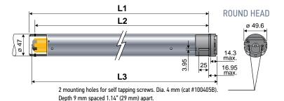
**Dimensions** 506 510 L<sub>1</sub> 25.7 in. (653 mm) 25.7 in. (653 mm) L2 25.2 in. (640 mm) 25.2 in. (640 mm) L3 SH 26.2 in. SH 26.2 in. (666 mm) (666 mm) RH 26.1 in. RH 26.1 in. (663 mm) (663 mm) 6.5 ft. (2 m) Cable Length 6.5 ft. (2 m)
